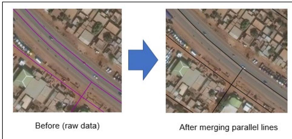
Figure 2. Shows the output of the road dataset after merging parallel lines such as motor ways.
