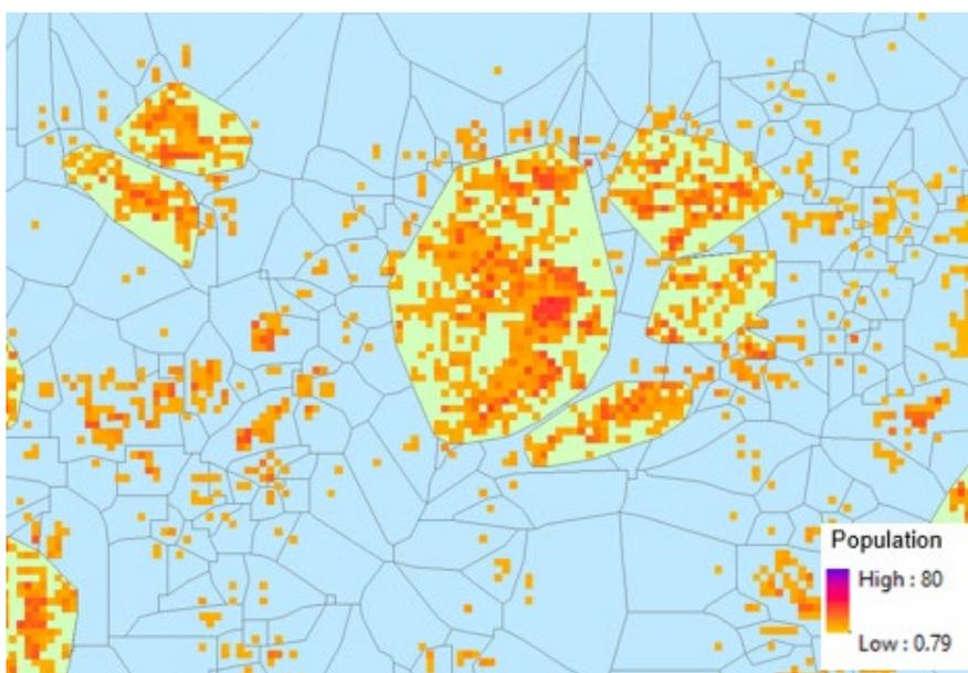
Figure 4. Example area showing full coverage adjacent polygons for BFA. The green colour represents polygons generated from convex hull techniques with a total population of 650 and higher. The blue colour represents the adjacent polygons generated from the Euclidean Allocation technique with a total population lower than 650.
